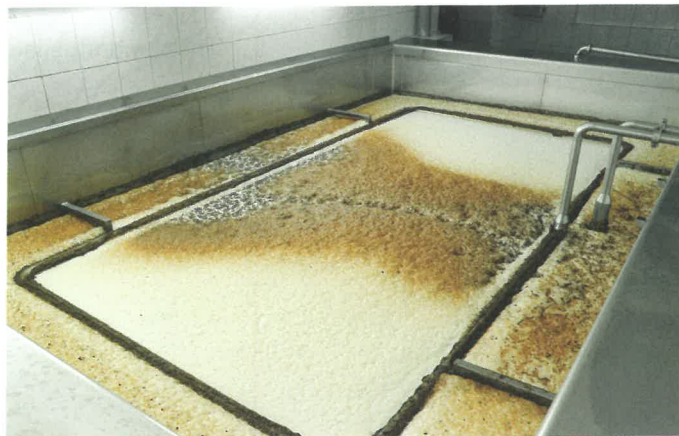
▲ Figure 21.3 A froth forming on the surface of the beer as yeast ferments the sugar to alcohol and carbon dioxide. The carbon dioxide in the froth prevents oxygen entering the mixture from the air – keeping conditions anaerobic.
