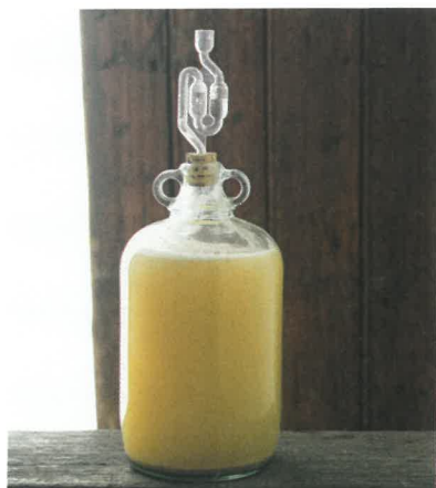
▲ Figure 21.2 A small fermenter for producing homemade wine. The U-shaped tube at the top is a water-filled airlock that prevents oxygen entering the fermenter but allows carbon dioxide to escape.
